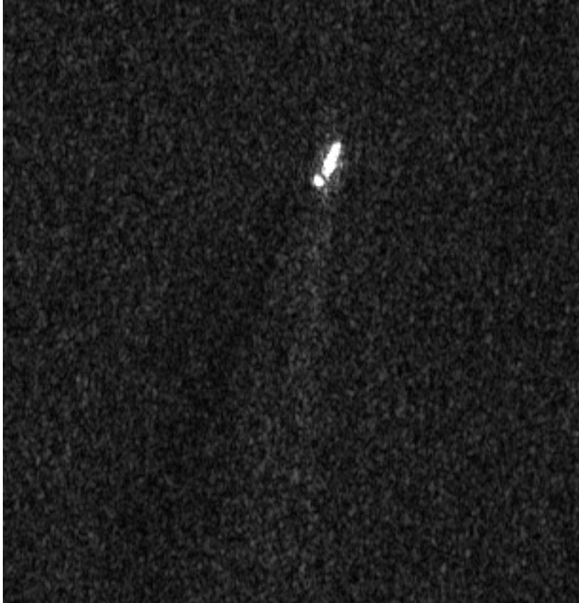
Figure 12.2c RADARSAT-1 (C-band, HH) Standard Mode image of a large ship showing some ship structure. Image was acquired on 5 November 1997 at 1111 UTC. The ship is located off the east coast of the U.S. near Chesapeake Bay. ©CSA 1997.
