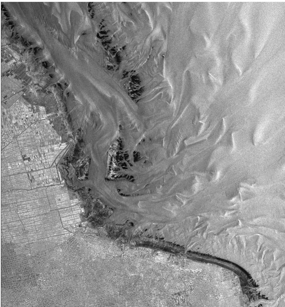
Figure 10.8. ERS-1 (C-band, VV) SAR image acquired 8 July 1995 showing the Xinchuan Gang (Subei) Shoal off the coast of China (north of Shanghai). The dark areas are sea areas that have fallen dry during ebb tide. (Also, because this image is not corrected for the variation of the image brightness with incident angle, the image intensity is high in the lower section of the image corresponding to near range [steep incident angles].) The imaged area is 100 km x 100 km. ©ESA 1995
