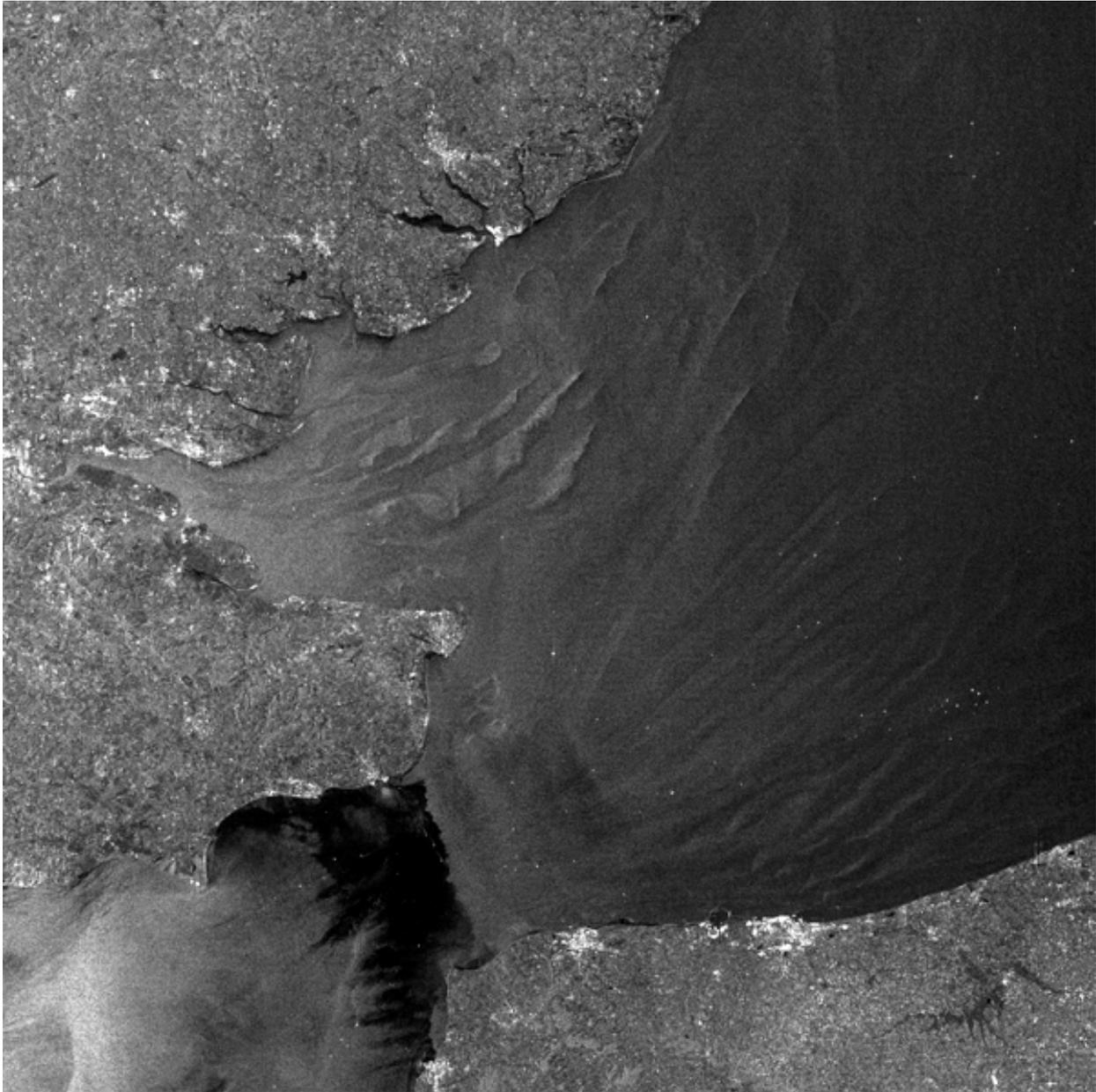
Figure 10.7. ENVISAT (C-band, VV) ASAR image of the Strait of Dover (English Channel) acquired on 21 August 2002. The image shows the English coast with the Thames estuary (upper left) along with a section the French and Belgian coasts (lower right). Underwater bottom features can be delineated east of the Thames estuary and north of the Belgian coast. ©ESA 2002
