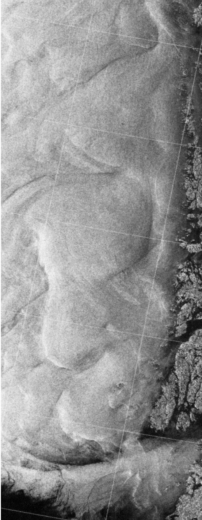
Figure 6.8. ERS-1 (C-band, VV) SAR image taken off the west coast of Norway on 3 October 1992. The bright/dark meandering linear features are signatures from strong current gradients that are perturbing the amplitude of the Bragg waves. The brightness of the signature (and whether it appears bright or dark) depends on the strength and orientation of the current gradient. The imaged area is 100 km x 300 km. ©ESA
